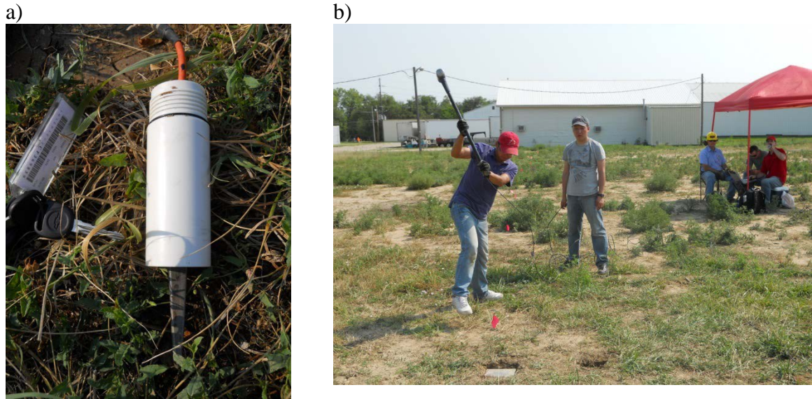
Figure 6.17 (a) borehole geophone potted in well-point PVC pipe, (b) MSOR impacts by 10 lb sledgehammer on aluminum plate
