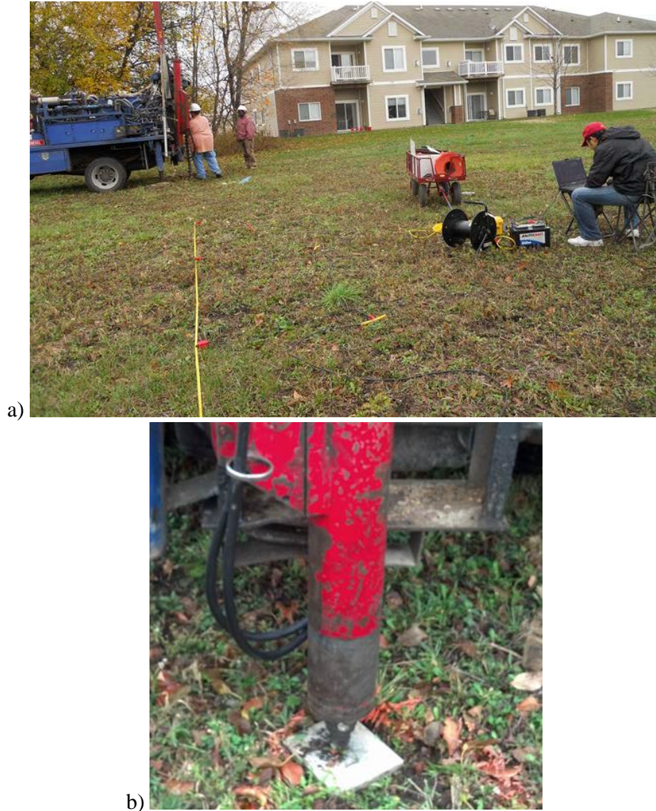
Figure 6.24 Preliminary MMSW-SPT test: a) SPT drill rig and geophone layout, b) SPT hammer impacting aluminum plate on the soil surface.
